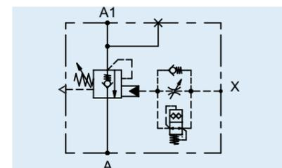
Single acting counterbalance valve with pilot signal dampening (Pat)
